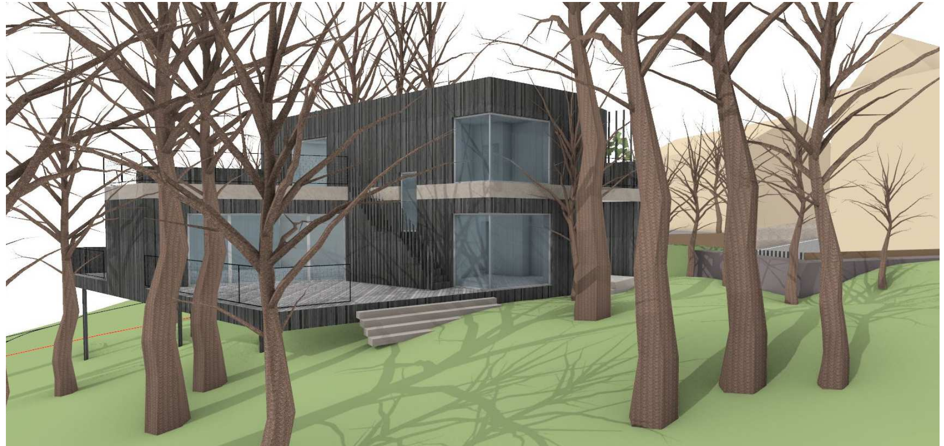
View from the southwest showing charred vertical timber cladding, textured lime render, wood decking and black stilts below.
