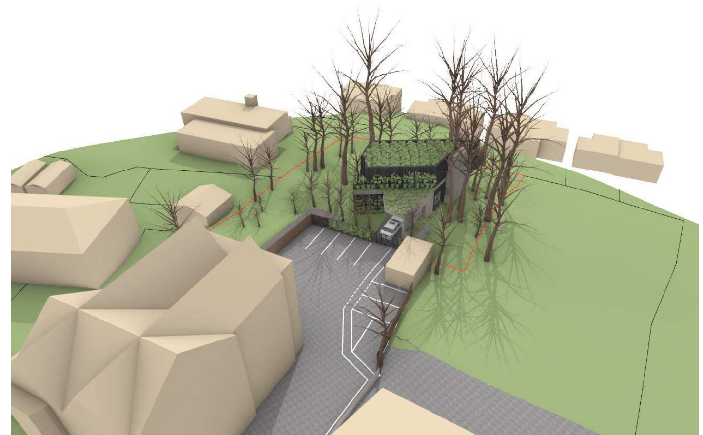
View from the north showing the planted roofs of the house and car port as well as the trellis wall on the north facade.
