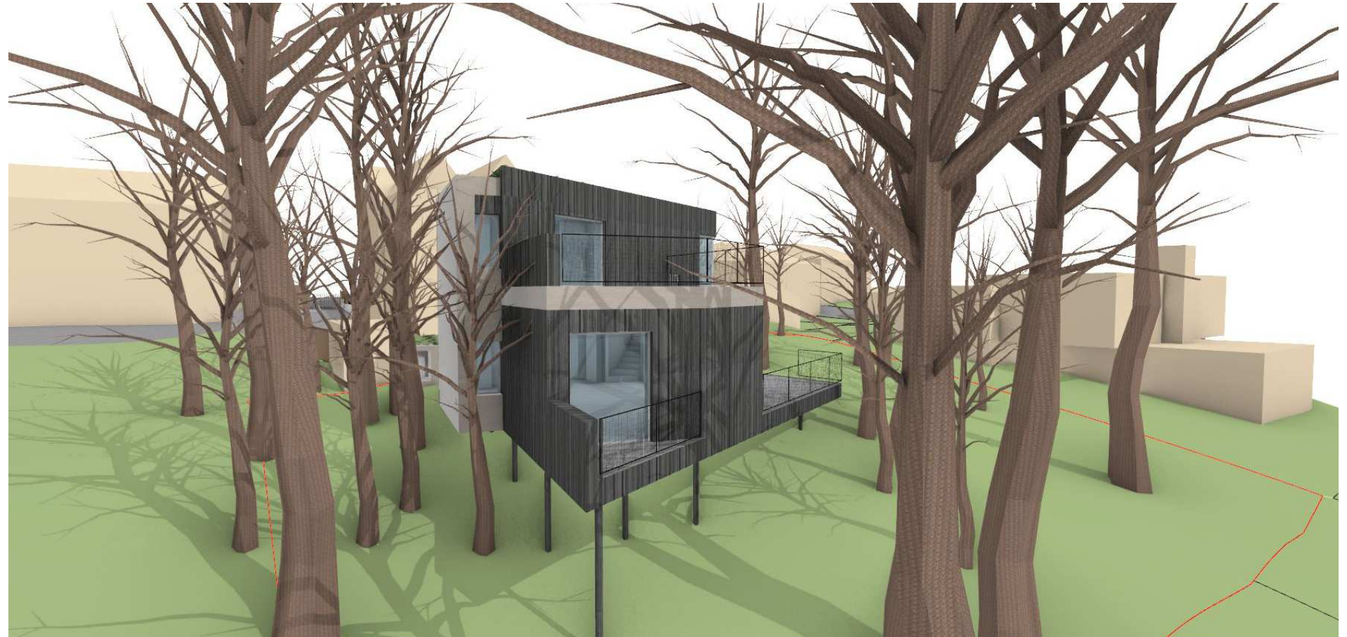
View from the southwest showing charred vertical timber cladding, textured lime render, black stilts below and black metal railings to outdoor decks.
