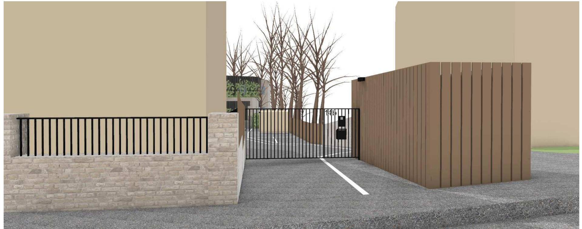
View from Highland Road showing new gate, intercom, post box, house number sign and lighting. Bin store is extended to the rear. Pedestrian striping added for wayfinding.
